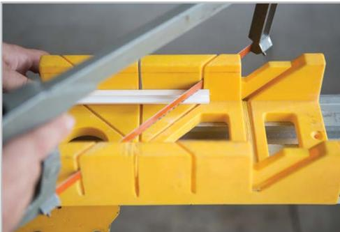
*Mitre the two lengths of F-Rail at a 45 degree angle so they meet in the corner.*
